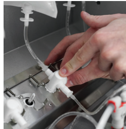
Lock the pump to the pump drive
