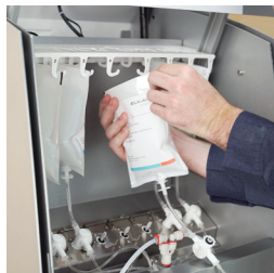
Insert the new pouch in the respective vacant slot by hooking it on the hanger
