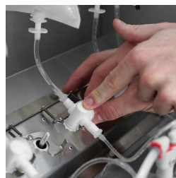
Lock the pump to the pump drive
