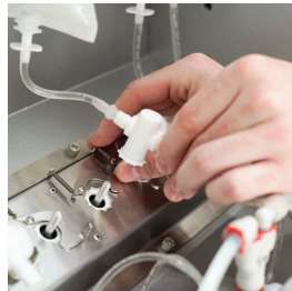
Unlock the silver pump clamp, popping out the pump
