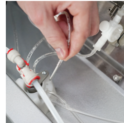
Insert the nib into the manifold
