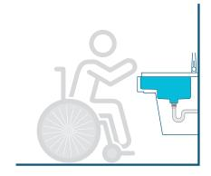
A raised work shelf at the front of the sink provides seated knee clearance. The back of the sink opens to an extra-deep 9" bowl for more space.
