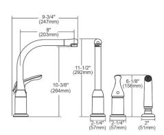
**Special Note:** 1.5 GPM flow regulator installed (2.2 GPM flow regulator also included with faucet)
