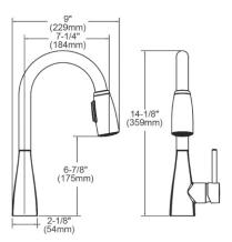
Special Note: 1.5 GPM flow regulator installed (2.2 GPM flow regulator also included with faucet)
