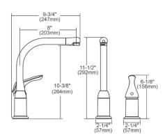
**Special Note:** 1.5 GPM flow regulator installed (2.2 GPM flow regulator also included with faucet)
