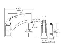
**Special Note:** 1.5 GPM flow regulator installed (2.2 GPM flow regulator also included with faucet)
