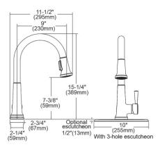
**Special Note:** 1.5 GPM flow regulator installed (2.2 GPM flow regulator also included with faucet)
