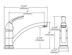
**Special Note:** 1.5 GPM flow regulator installed (2.2 GPM flow regulator also included with faucet)
