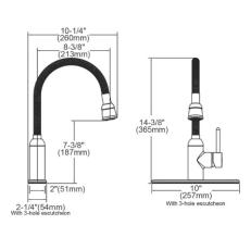
Includes: 1.5 gpm flow regulator installed (2.2 gpm flow regulator also
