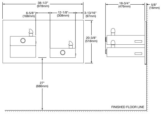
\*A.D.A. Compliant (24" [610mm] for Child A.D.A.). Adjust other measurements accordingly.
