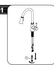
Shut off water supplies. Before installation, remove quick connect assembly (1) from the free end of pull-down hose.
