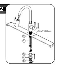
Retract pull-down hose (1) up through faucet body, until the pull-down hose fitting is flush with the bottom of shank (2). Do not pull hose fitting past the shank. Insert faucet body through the hole in sink. From underneath sink, install plastic washer (3), metal washer (4) and nut (5) onto the mounting shank. Do not overtighten. Note: Do not feed the pull-down hose (1)
