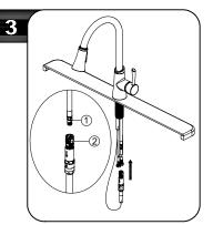
Screw quick connect assembly to the free end of pull-down hose. Align male fitting (1) and tabs (2) on quick connector. Push quick connector housing firmly upward and snap onto receiving male fitting. Pull down moderately to ensure connection has been made.
