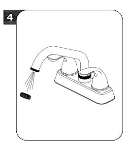
Important: After installation is completed, remove connector. Turn on water supply and allow both hot and cold water to run for at least one minute each. While water is running, check for leaks. Replace connector.
