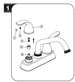
Shut off water supply. Remove set screw plug (1). With valves in "closed" position, unscrew set screw (2) and remove handle (3) from valve stem (6). Remove screw (4) and pull off adapter (5).
