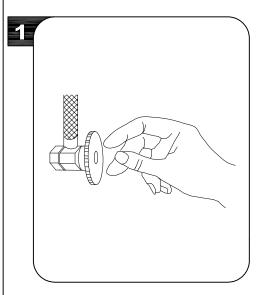
Shut off water supply at angle stop. Remove old faucet.Clean sink surface in preparation for new faucet.
