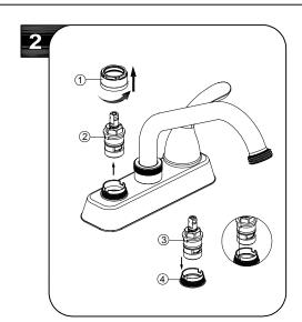
Loosen sleeve (1) by turning it counter-clockwise and lift out the cartridge (2). Remove old cartridge and replace with new cartridge. Make sure the wings (3) on the two sides of the cartridge sleeve fit well into the slots (4) on the body. Tighten sleeve (1). Reinstall the handle.
