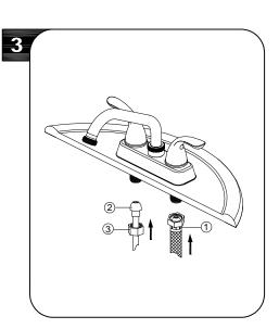
Make connections to water lines. Use 1/2" IPS faucet connections (1) or use coupling nuts (3) with 3/8"O.D.ball-nose risers (2). Use wrenches to tighten connections. Do not overtighten.
