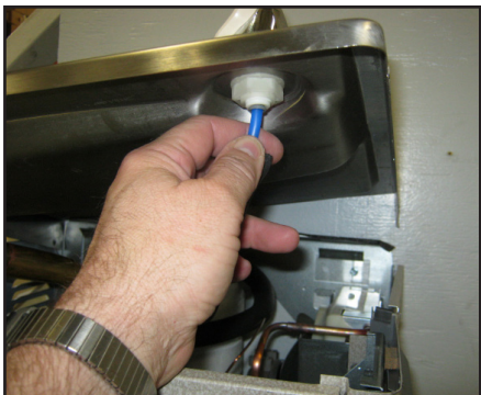
Remove Bubbler Water Line
