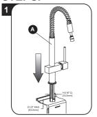
Before inserting the single lever group in the hole of the sink, make sure that the base gasket is properly positioned in its seat and that the flexible hoses are well tightened to the body of the tap.
