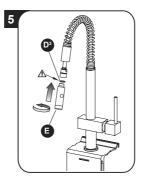
Tighten the shower (E) to the hose interposing the gasket (D3) and confirm the hose can slide smoothly through the passage hole.
